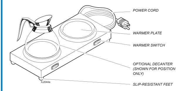
Fig. 1 Features & Operating Controls
